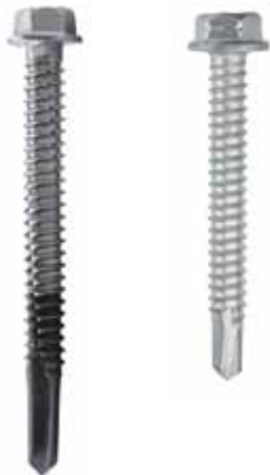
Bi-metallic fasteners are also selectively-hardened. The drill-tip and tapping threads are high-carbon steel, fused to a stainless steel shank (left, before coating). The high-carbon steel is hardened, leaving the shank unaffected. The entire fastener is then covered with corrosion-protective/galvanic barrier coating (right). Courtesy of Elco Construction Products.
