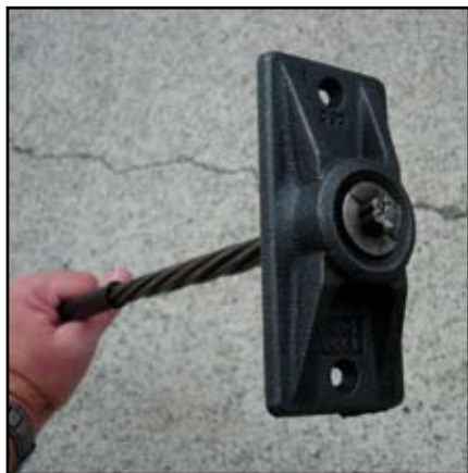
Figure 1: Standard Post-Tensioning 7 Wire Strand and Anchor.
