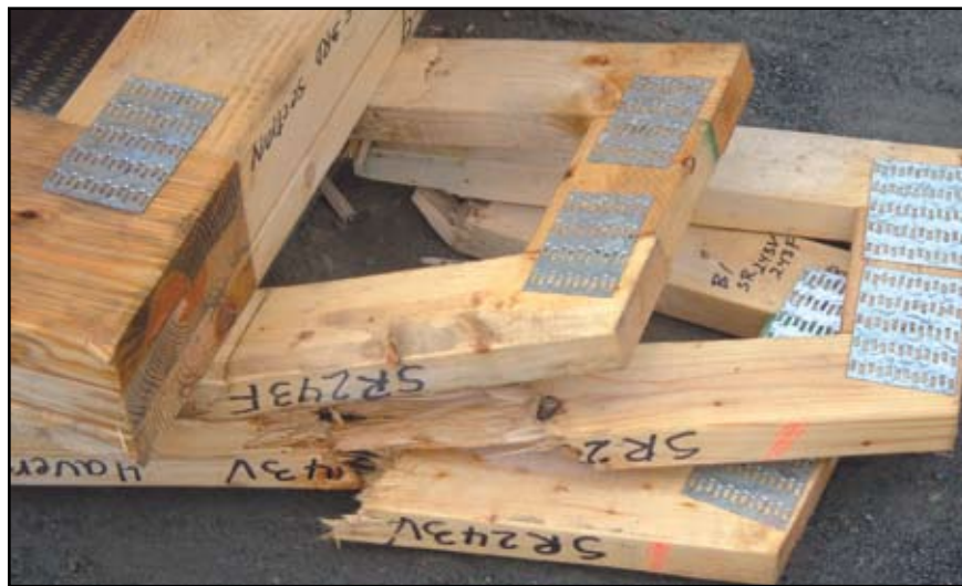
Figure 2: Damage to the ends of three trusses resulting when additional trusses were dropped on top of them during delivery.
