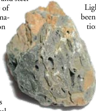
Figure 1: Lightweight aggregate particle showing ceramic matrix and void structure.
