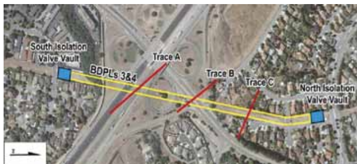
Figure 2. Hayward Fault Traces A, B, and C. Courtesy of URS Corporation.
