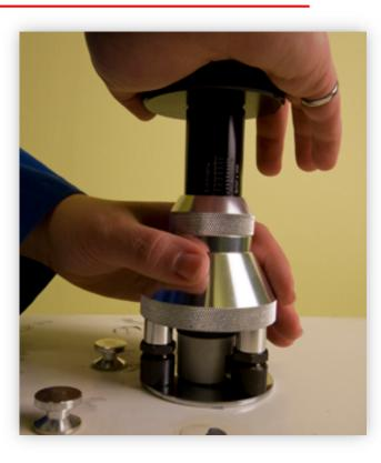
• ASTM 7234 Pull Off Adhesion Strength of Coatings on Concrete, a test bias becomes a factor as a result of the various pull off testing apparatus that is used.
