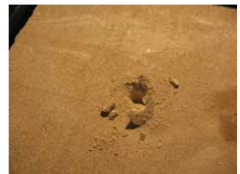
Figure 4: Tension failure modes: small cone (upper left), cube splitting (upper right), face delamination (lower left), anchor pull-out (lower right).
