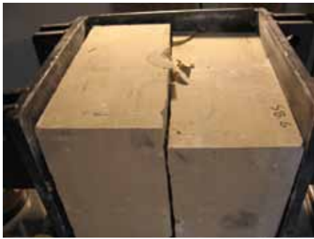
Figure 5: Sandstone specimens that failed by cube splitting.
