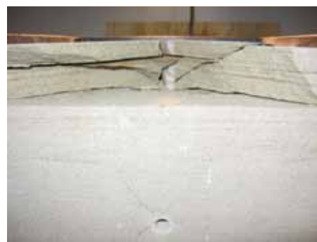
Figure 4: Tension failure modes: small cone (upper left), cube splitting (upper right), face delamination (lower left), anchor pull-out (lower right).
