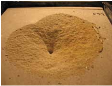
Figure 3: Tension failure modes: large cone (left) and bolt fracture (right).
