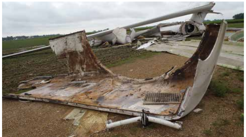
Figure 4. Localized debris field following wind turbine over-speed, due to mechanical failure within the nacelle. Remnants and evidence were found 650 feet (198 meters) from the tower base.
