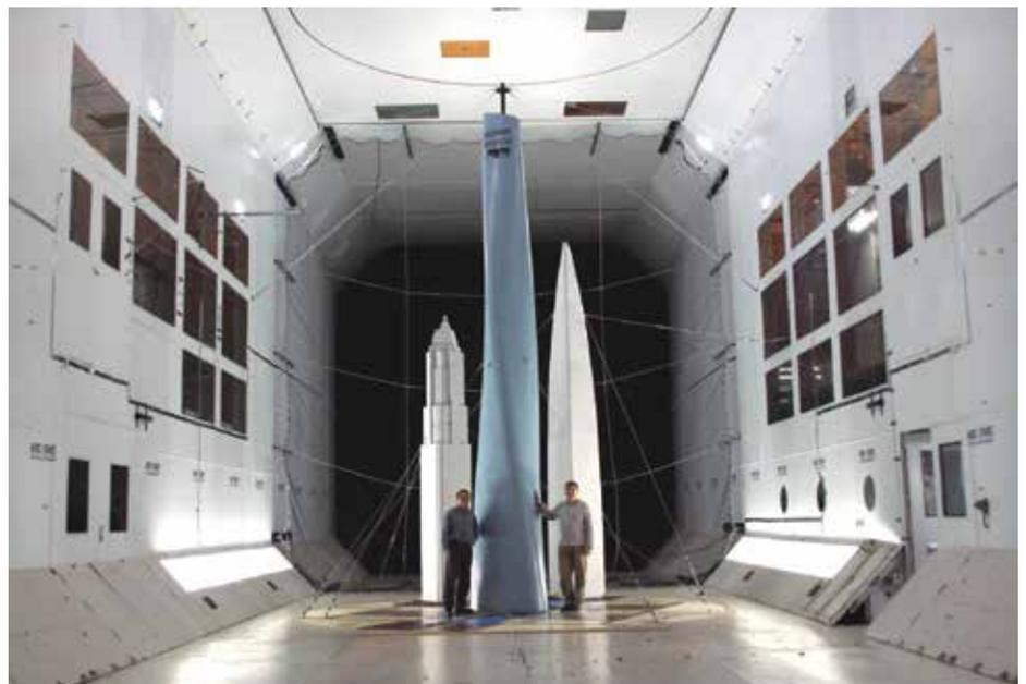
Figure 4. Large scale wind tunnel testing of the Shanghai Tower. The final design has a 180-degree twist as it rises and its base is rotated to be aerodynamically efficient in the direction of the strongest winds.
