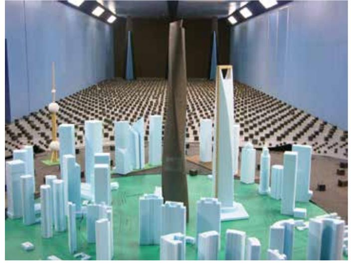
Figure 3. One of the prototype shapes that was explored for the Shanghai Tower before selecting the final design. This option has a 180-degree twist as it rises.
