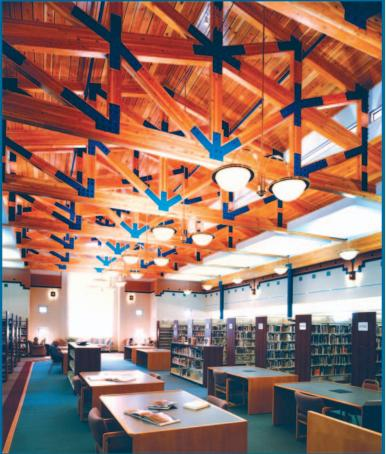
The architect and contractor note that the timber framing gives a warm rustic appearance and saves money, because steel trusses would "...a warm rustic have been shop-fabricated and would require more time to assemble than wood. appearance..."
