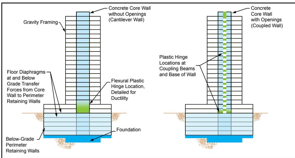
Figure 2: The typical nonlinear action for a cantilever wall (left) is a flexural plastic hinge at the base of the wall. For a coupled wall (right) nonlinear actions are flexure-yielding coupling beams and a flexural plastic hinge at the base of the wall.
