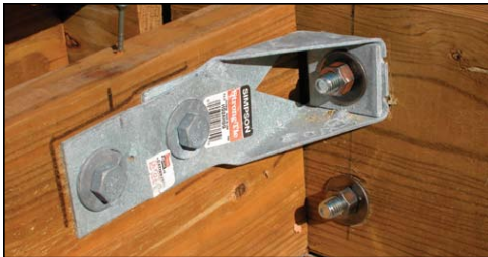
Figure 3: Simpson Strong-Tie™ HD2A connector used to test an assembly with the post inside band joist (shown) and outside band joist.
