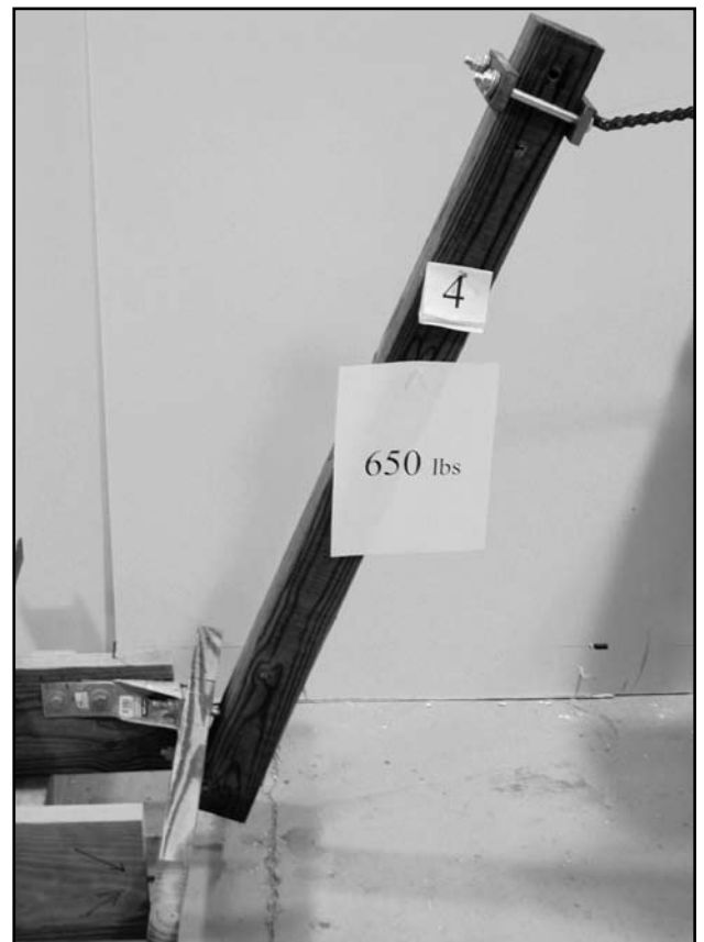
Figure 6: Outside band joist specimen loaded with 650 pounds. The specimens exhibited extreme “ductility” and this test characteristic is considered a desirable safety feature.
