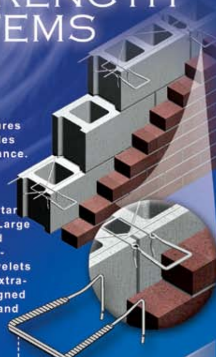
Pintles are flattened and serrated for superior bonding with mortar.
