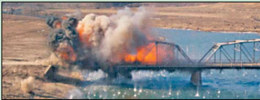
Explosive testing of a steel truss bridge
