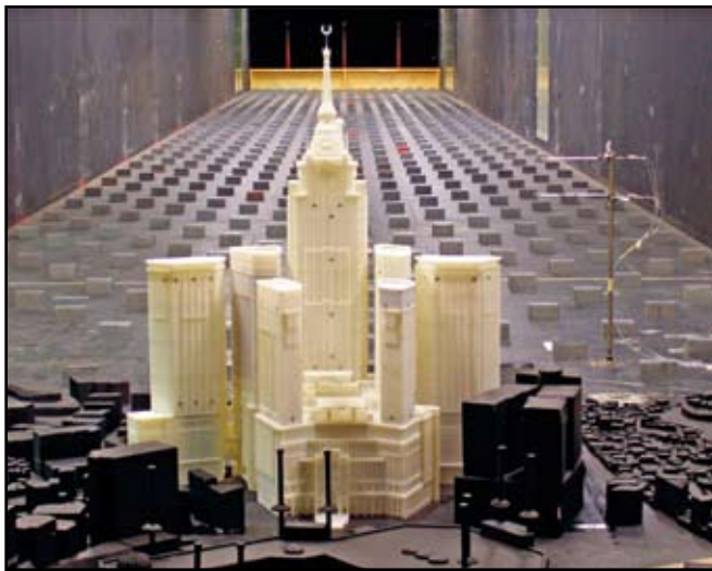
The Development of King Abdul Aziz Mekkah in the wind tunnel. Pressure model of 7 towers, 5 of them sitting on top of an extensive podium. Structural loads were determined by integration of local pressure measurements over all surfaces of the buildings.
