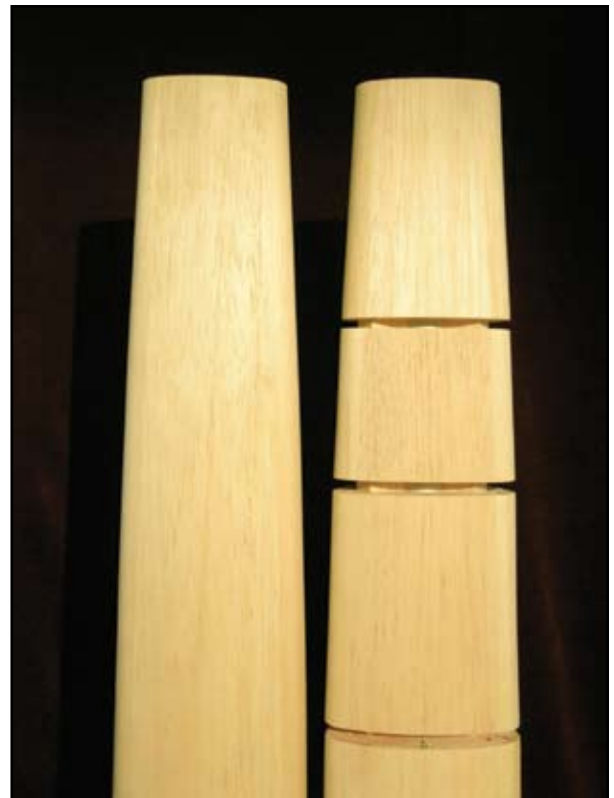
Example of refuge floors and skygardens being opened to reduce response
