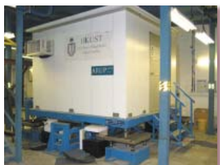
Figure 3: Simulated Office Environment at HKUST Low Amplitude Shake Table (© Arup)
