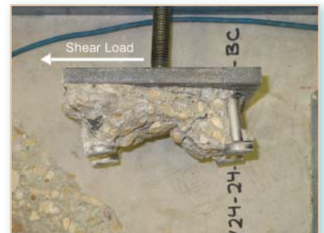
Figure 11: Photograph of pryout failure for a four-stud group
