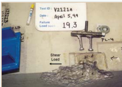
Figure 7: Side-edge concrete breakout when the shear force is applied parallel to the free edge
